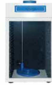
Soundproof box chamber with lifting platform
