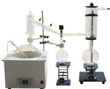
Short-path distillation can be widely used in all aspects of the national economy, especially suitable for the separation of high boiling point, heat sensitive and easily oxidized materials. Nowadays, the short path distillation has been applied in the following fields successfully.
