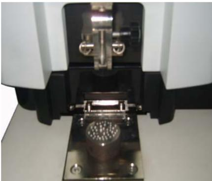
8. The CX-9800 spectrometer has a compact design for the incident light path. By connecting the incident light path directly to the vacuum system, the two lenses separate the entrance window from vacuum and dust protection, making maintenance easy and convenient for customers to carry out in their daily work.
